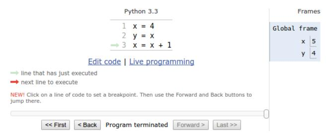
**Figure 3:** Watching code run in the Python Tutor visualization tool. Final values are presented on the right under the label "Global frame." Use the buttons "First," "Back," "Forward," and "Last" to visualize each step of your program.
